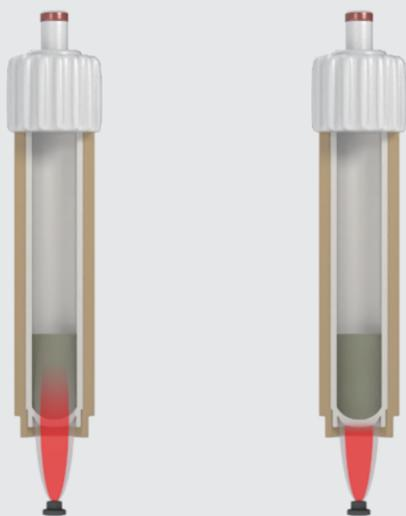
Rtemp sensor's excellent IR penetration of TFM wall allows temperature of the digestion solution being detected directly
